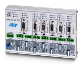
The ProfiHub B5+RD is identical to the regular ProfiHub B5 family. However, it is equipped with an additional integrated micro ProfiTrace diagnostic unit. The ProfiHub offers a PROFIBUS DP slave device to transfer bus statistics and device event information to the PLC/DCS system. This allows you to reduce unexpected downtime to a minimum. This solution has the following unique features:
